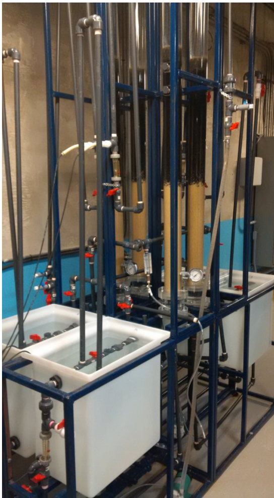
Figure 4: Biofiltration pilot, consisting of four small-scale filtration columns.
